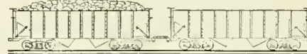
Loaded Car, 150,000 lbs. Empty Car, 40,000 lbs. Braking Power Braking Power 60% on 50 lbs. cyl. pres. 60% on 50 lbs. cyl. pres. Draw Bar Strain 4,040 Lbs.
